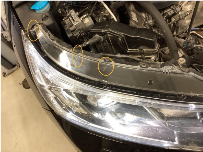
2.1 Krakelering i plast
