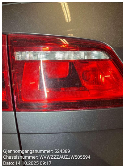
2.1 Krakelering i plast
