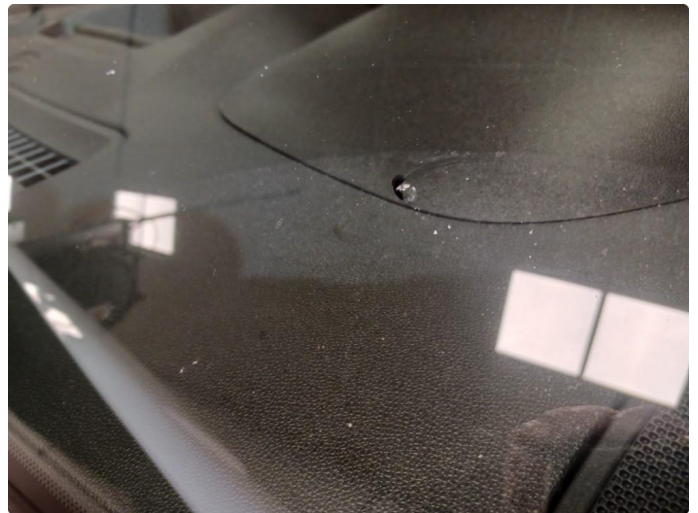
1.2 Steinsprut i synsfelt
