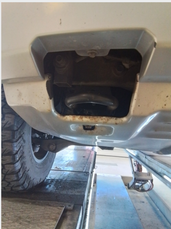
2.2 Rust bunnplate motor
