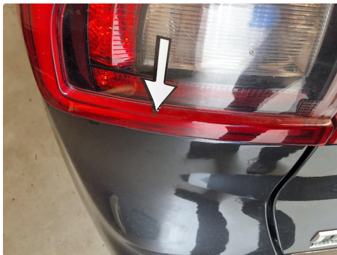
2.1 Krakelering i plast
