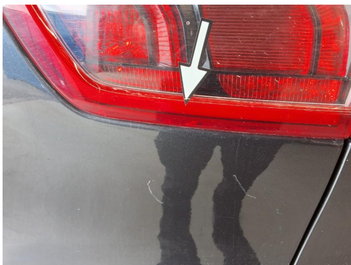
2.1 Krakelering i plast
