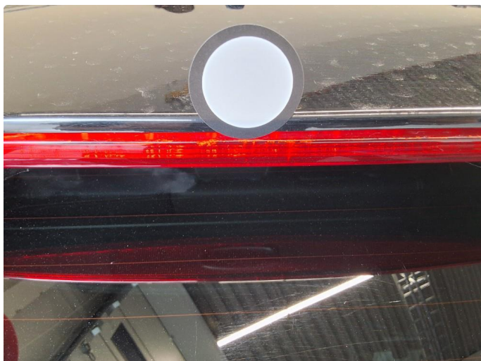
2.1 Krakelering i plast
