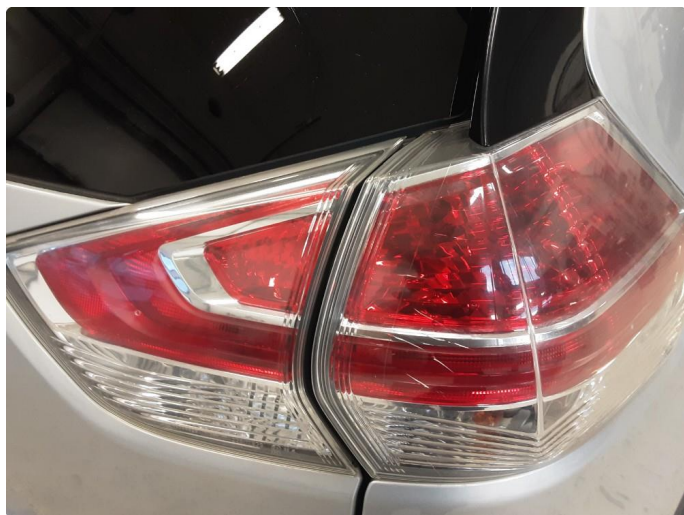
2.2 Krakelering i plast
