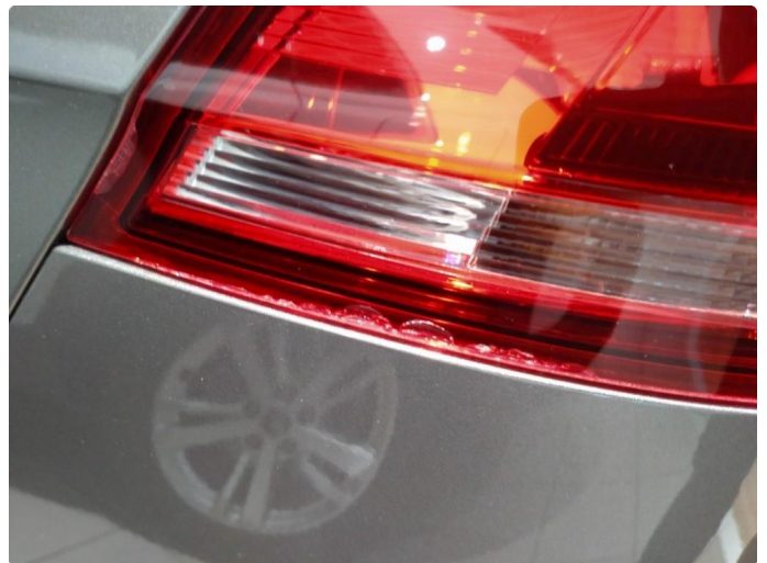
2.1 Krakelering i plast
