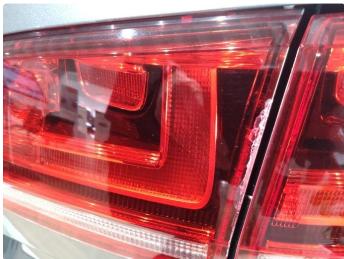
2.1 Krakelering i plast
