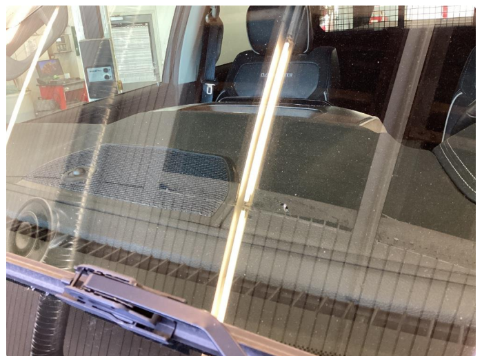
1.3 Steinsprut i synsfelt
