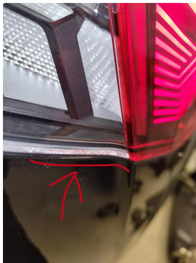
2.1 Krakelering i plast
