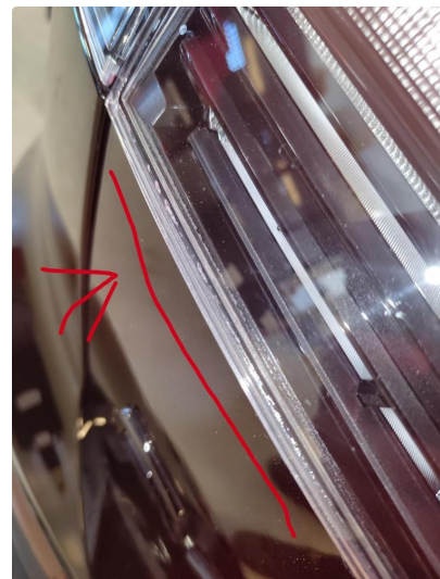
2.1 Krakelering i plast
