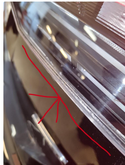
2.1 Krakelering i plast
