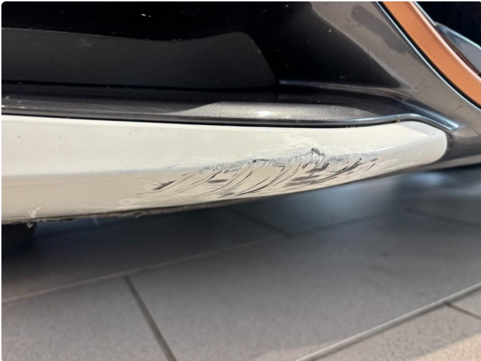
1.1 Oppskrapet under frontfanger v.leppe v.side
