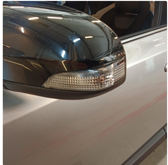
2.2 Sprekker i blinklys glass
