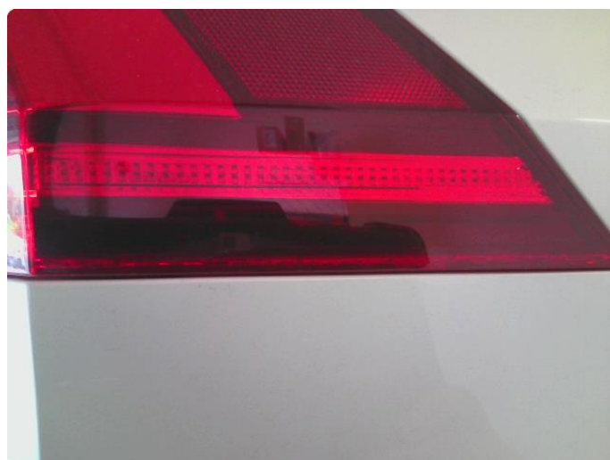
2.1 Krakelering i plast
