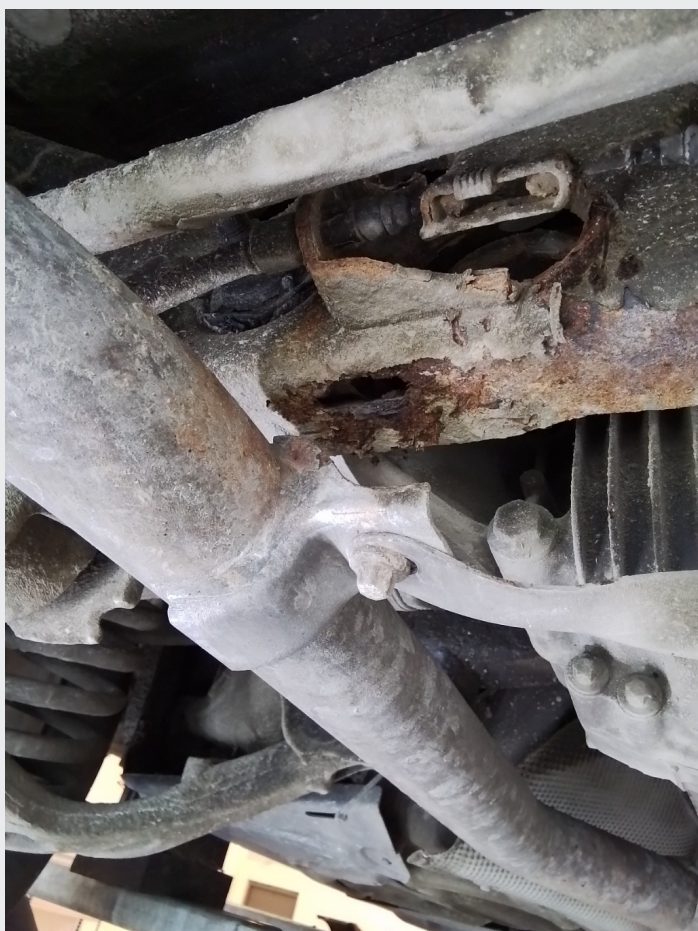
8.5 Opprustet travers (rusthull)
