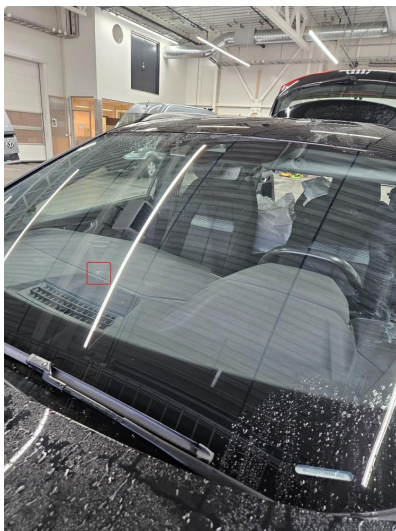
1.2 Steinsprut utenfor synsfelt - reparert/limt, anmerket for info
