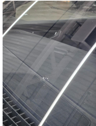
1.2 Steinsprut utenfor synsfelt - reparert/limt, anmerket for info
