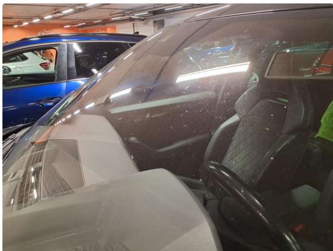
1.7 Steinsprut i synsfelt
