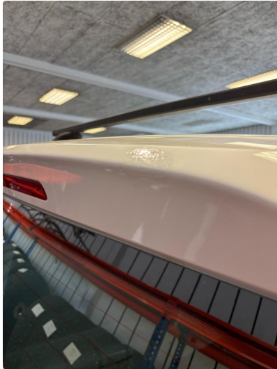
1.2 Lakkert over lakkskade
