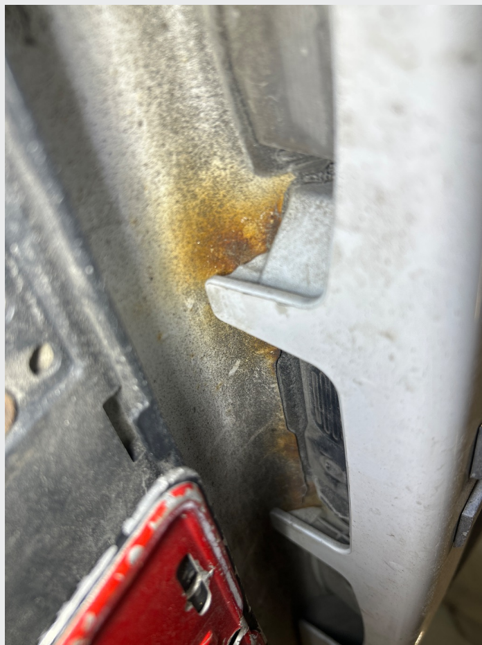
2.5 Rust i bakluke
