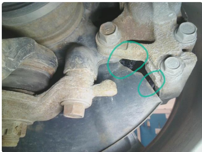
2.2 Mer enn 25% rust
