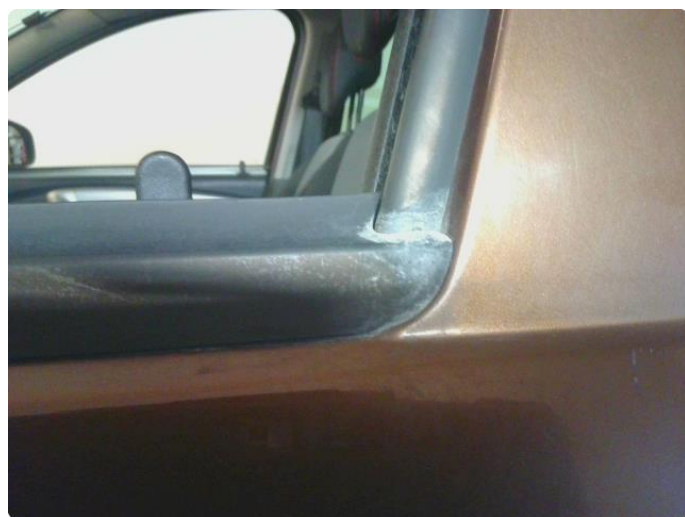
2.6 Rust under list
