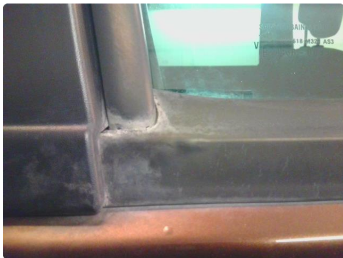
2.6 Rust under list
