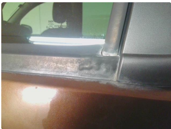
2.6 Rust under list
