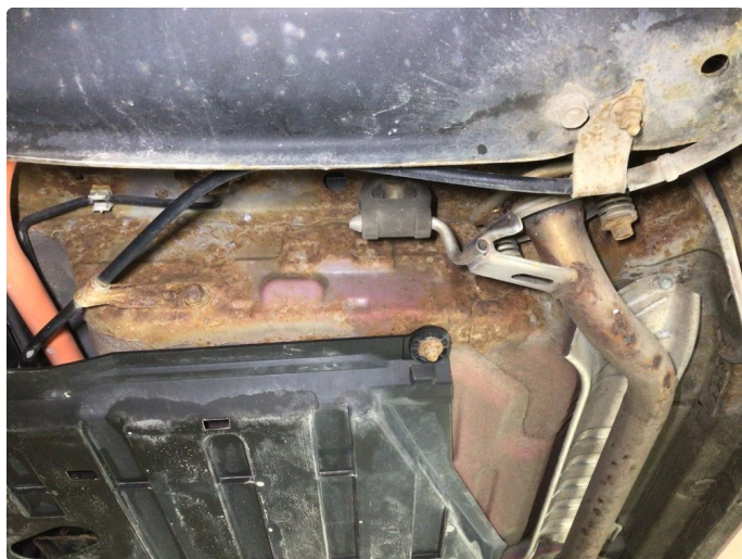
4.2 Overflate rust under bil
