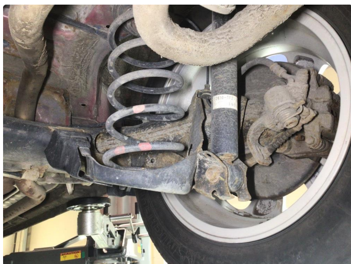
4.2 Overflate rust under bil
