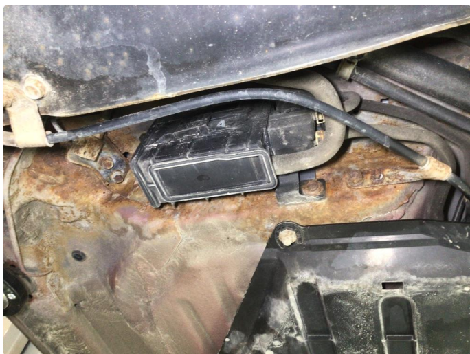
4.2 Overflate rust under bil
