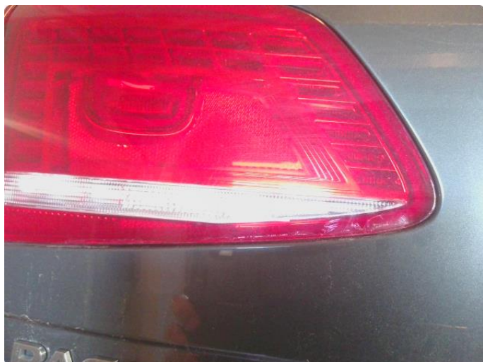
2.2 Krakelering i plast
