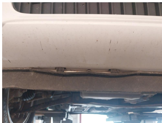
1.16 Skrubbskader under frontfanger, løs list under frontfanger
