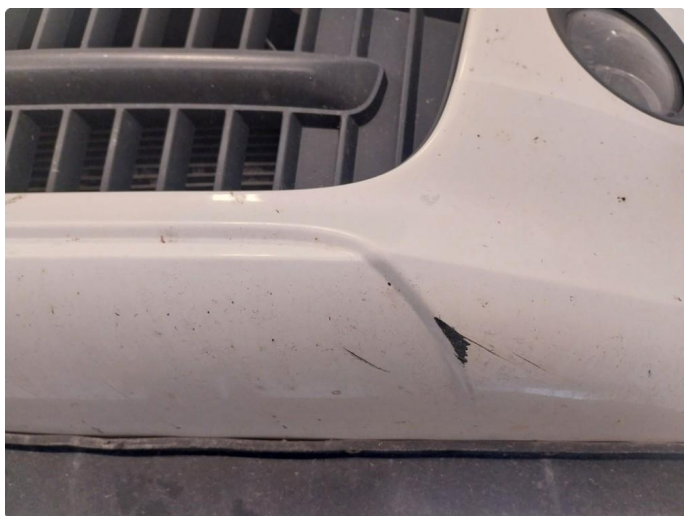
1.16 Skrubbskader under frontfanger, løs list under frontfanger
