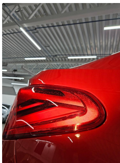
2.1 Krakelering i plast
