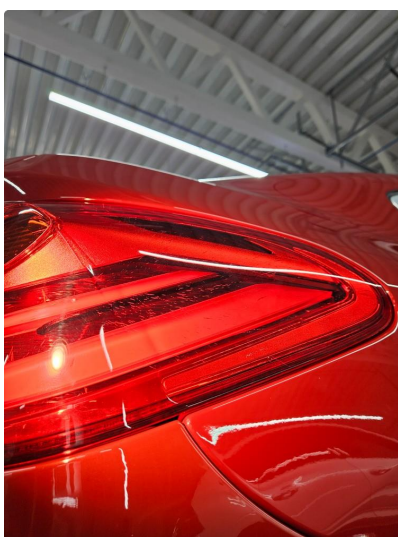
2.1 Krakelering i plast
