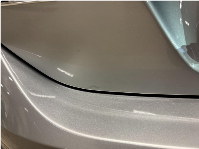
1.1 Liten rustblemme under lakk
