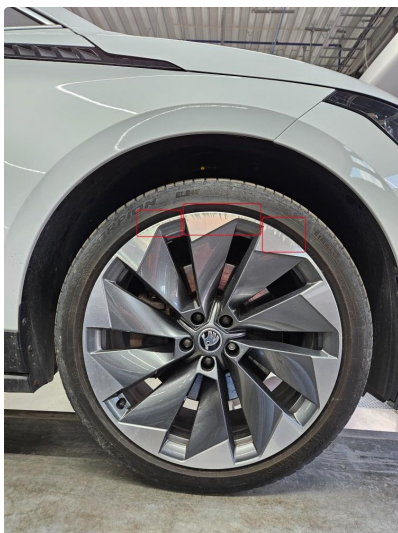
1.1 Noe riper/skrubbemerker, h.side foran
