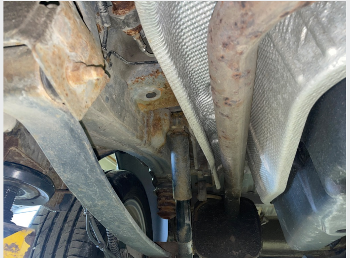
2.2 Litt overflate rust
