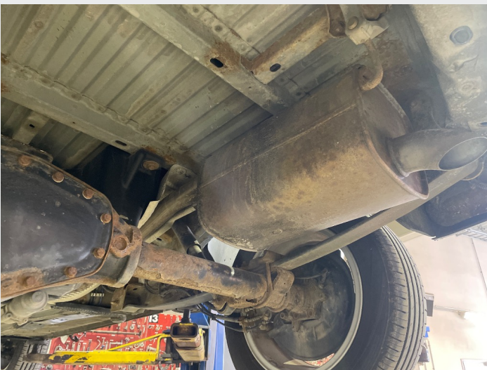
2.2 Litt overflate rust
