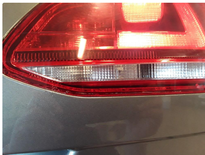
2.2 Krakelering i plast.
