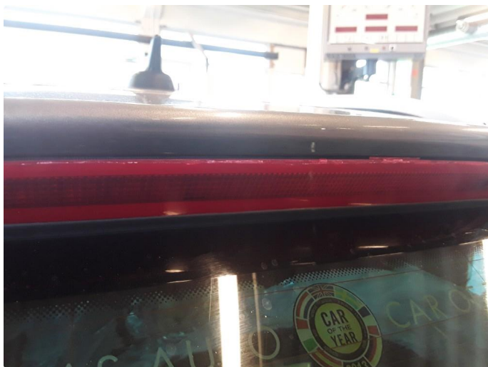
2.3 Krakelering i plast.
