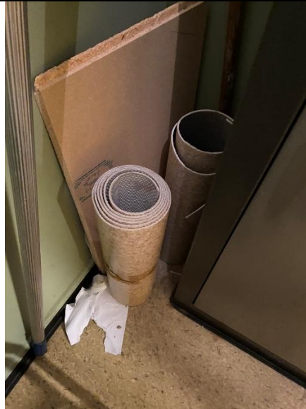
Plassering: Vent.rom Materialtype: Vinylgulvbelegg i ruller
