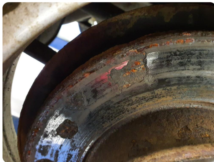
6.1 Mer enn 25% rust
