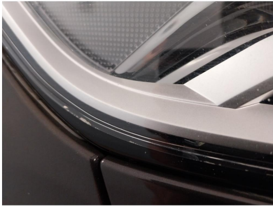
2.1 Krakelering i plast
