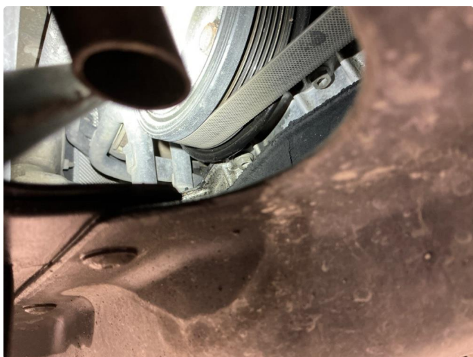
2.1 Oljesvetting bakkant motor.
