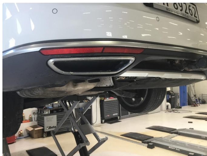
1.7 Bakfanger skadet underkant
