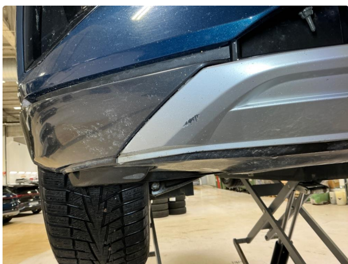
1.7 Fanger foran,skrubbskader underkant
