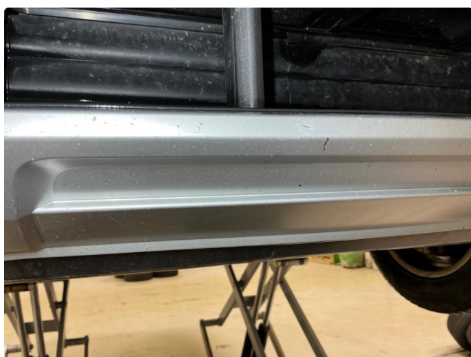
1.7 Fanger foran,skrubbskader underkant
