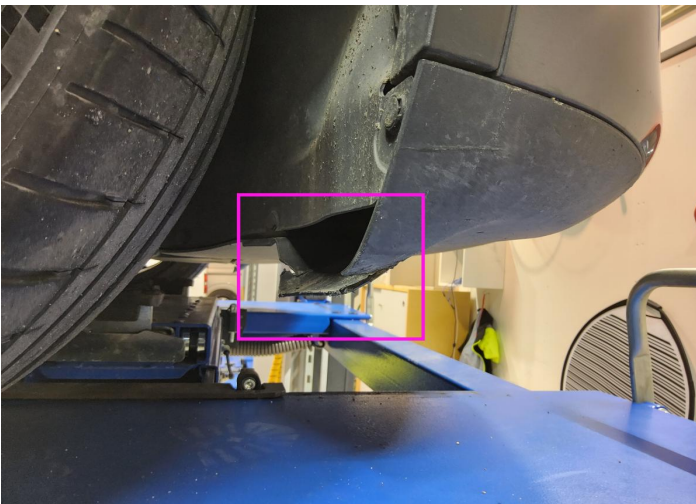
15. Bumper / Front Bodywork / Dent / Deformation -
