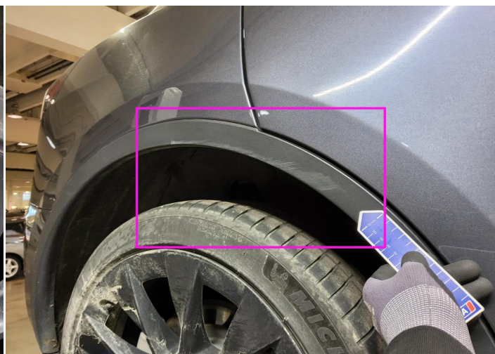
8. Fender / Back Right Paint / Scratch / Scuff -
