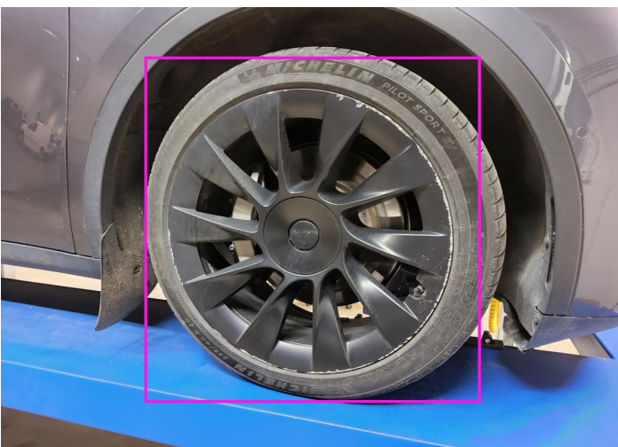
5. Rim / Front Right Out of Bodywork / Scratch -
