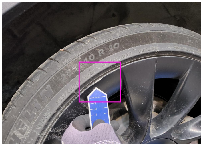
7. Rim / Back Left Out of Bodywork / Scratch -
