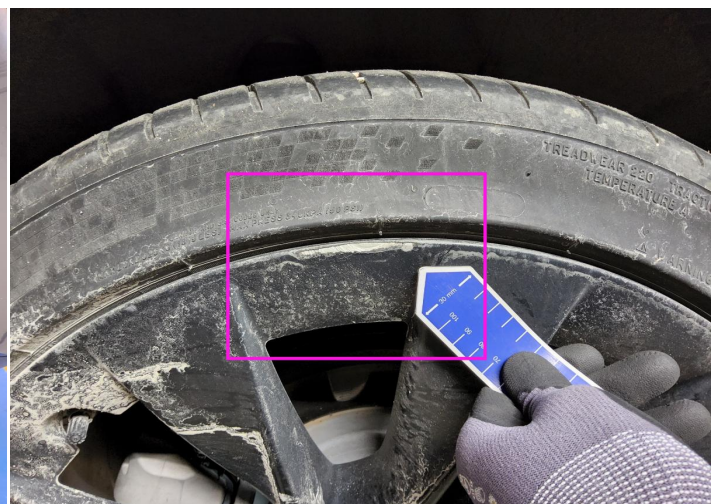
6. Rim / Back Right Out of Bodywork / Scratch -
