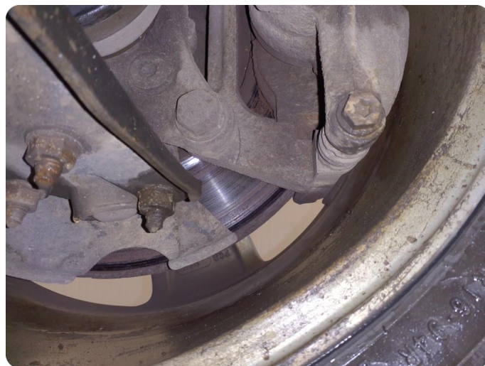
6.1 Slitte/stor slitekant Tillegg rust bremses bak
