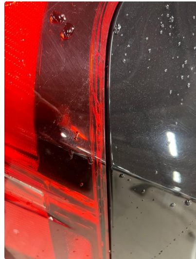
2.1 Krakelering i plast
