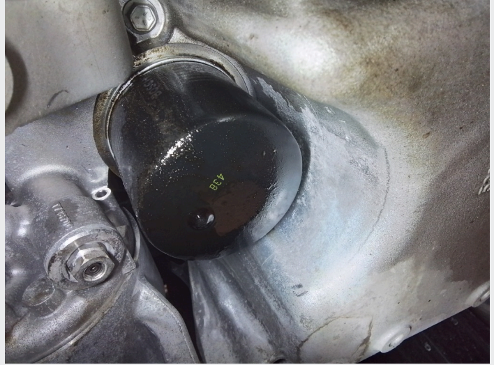
6.3 Svetting/lekkasje oljefilter motor
