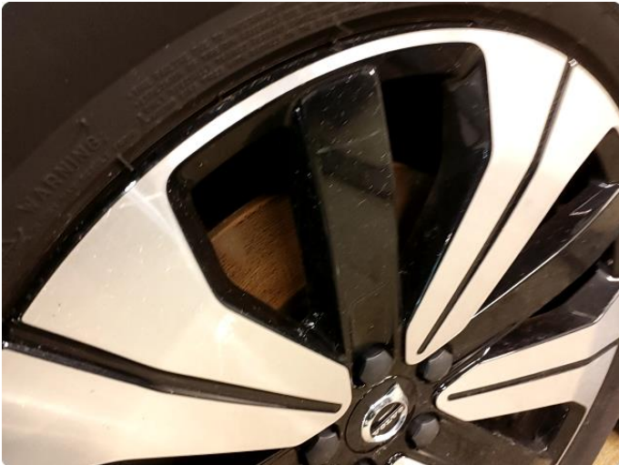
2.1 Mer enn 25% rust
