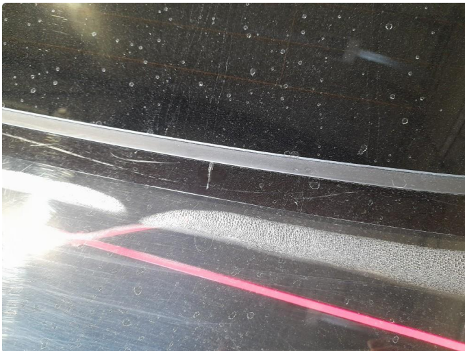
2.1 Krakelering i plast
