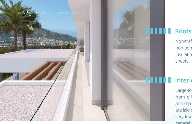
Non-trafficable flat roof, with heavy gravel protection, non-adhered waterproofing membrane, including thermal insulation by means of rigid extruded polystyrene foam sheets.
