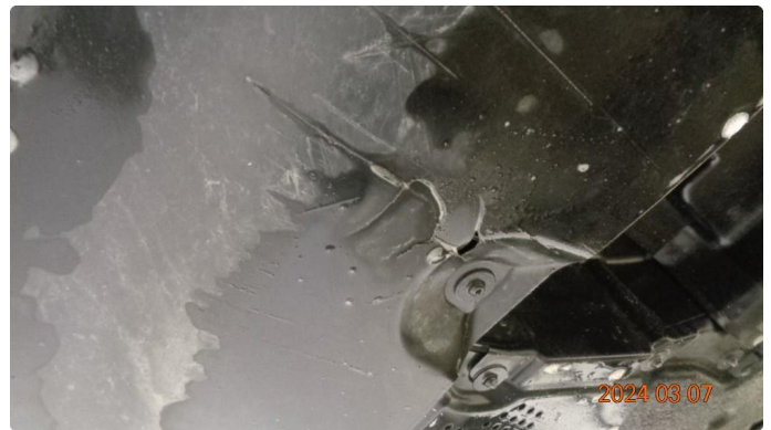
1.1 Sprukket plate under motor
