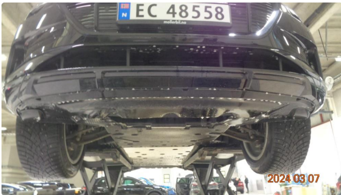
1.1 Sprukket plate under motor
