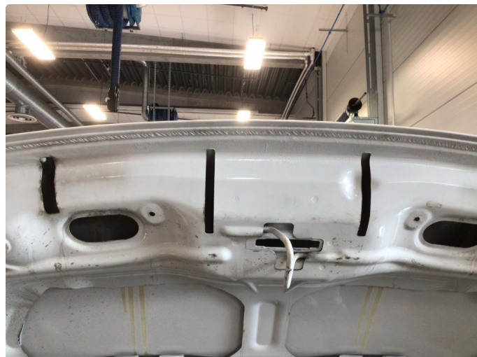
1.2 Rust i fals
