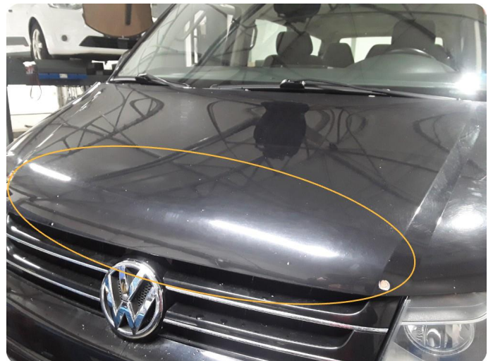
3.3 Steinsprut -ink rust
