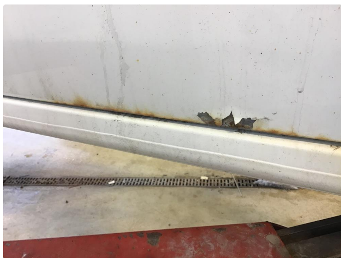
1.2 Rust i fals
