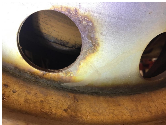
4.2 Mer enn 25% rust
