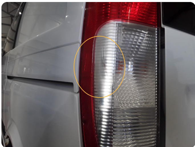
4.3 Defekt / sprukket glass
