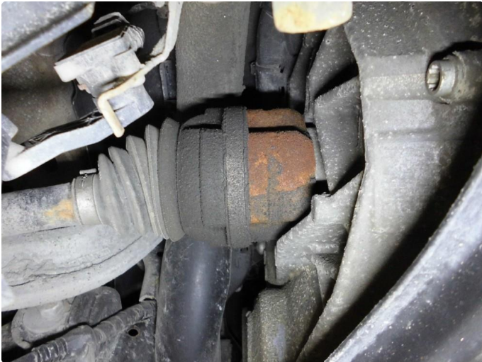
2.1 Noe svetteing rundt indre ledd venstre drivaksel bak / diff. bak
