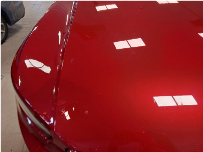
1.1 Panser lakkert pga steinsprut
