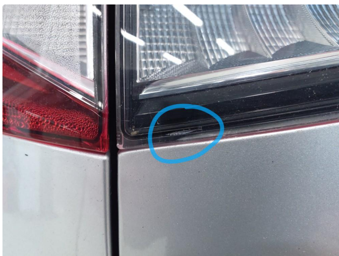
2.2 Krakelering i plast
