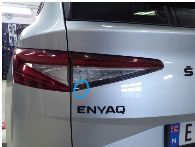
2.2 Krakelering i plast
