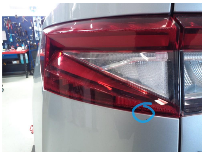
2.1 Krakelering i plast
