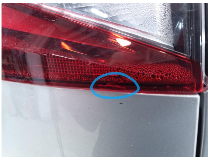
2.1 Krakelering i plast
