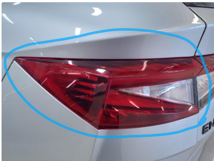
2.1 Krakelering i plast
