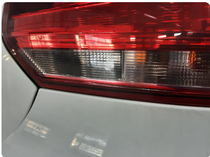
2.2 Krakelering i plast
