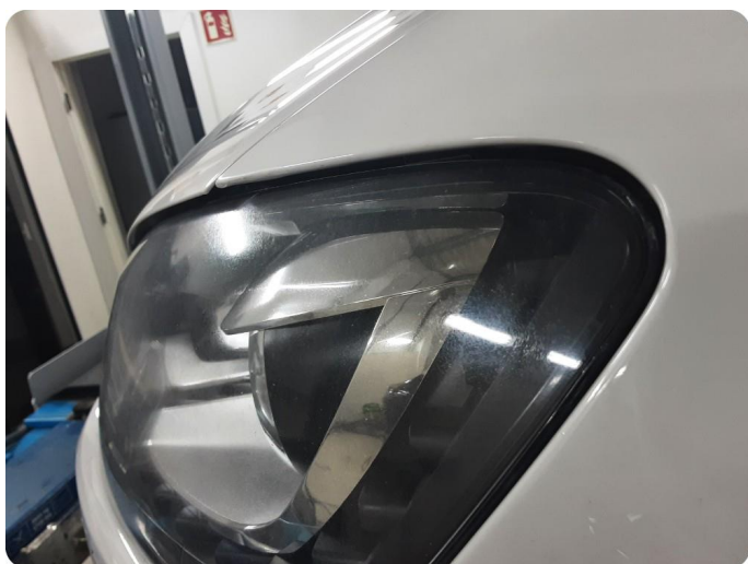
2.1 Krakelering i plast
