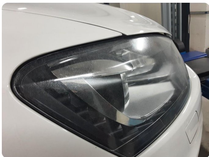
2.1 Krakelering i plast
